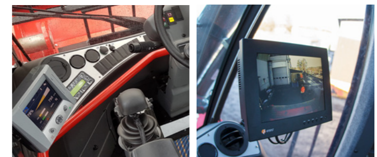
Red device bar for mounting various equipment like displays is optional for RTD1723 and RTD3126.
