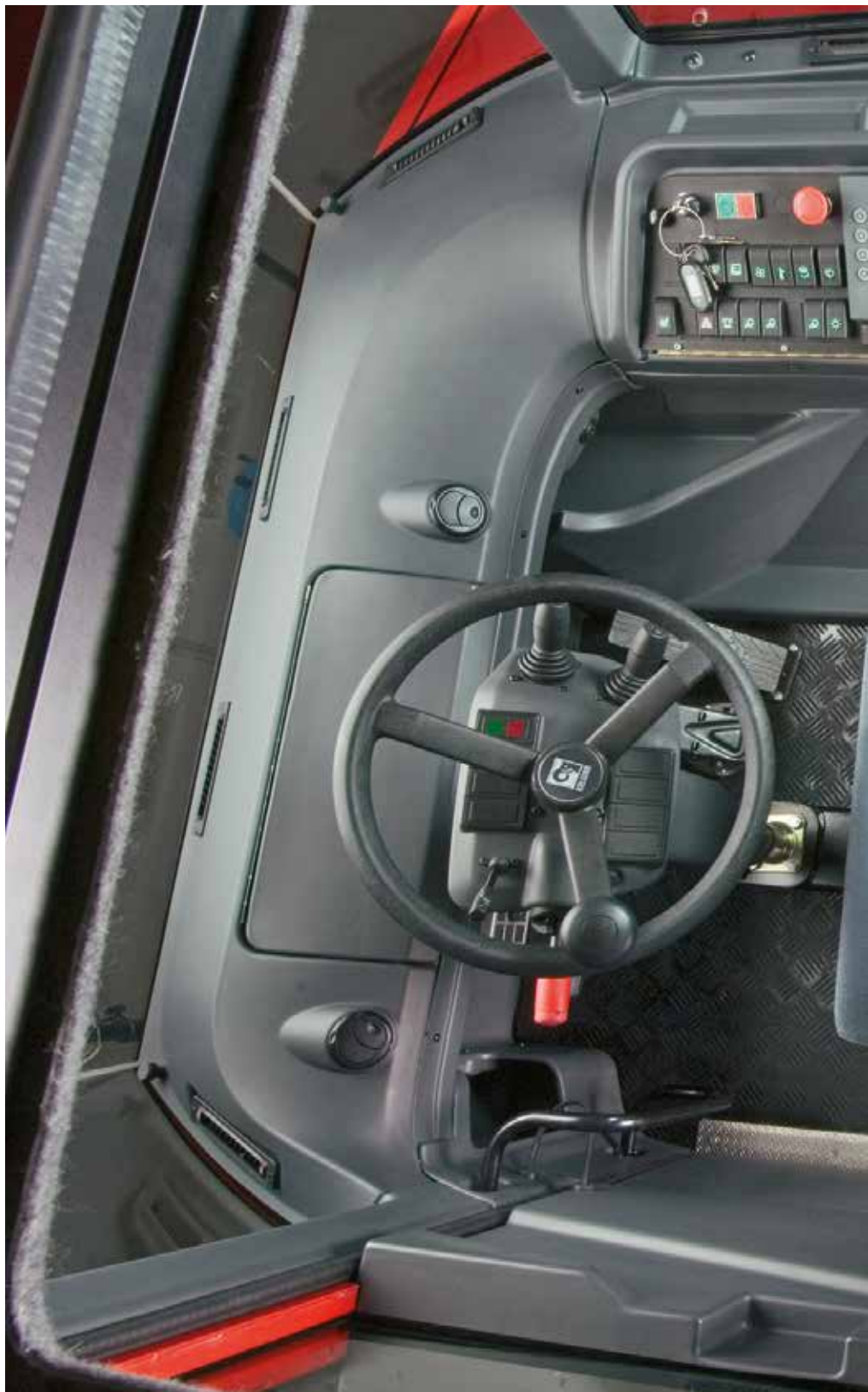
The wide-opening side door enables easy movement. The sturdy handles facilitate safe entry.
